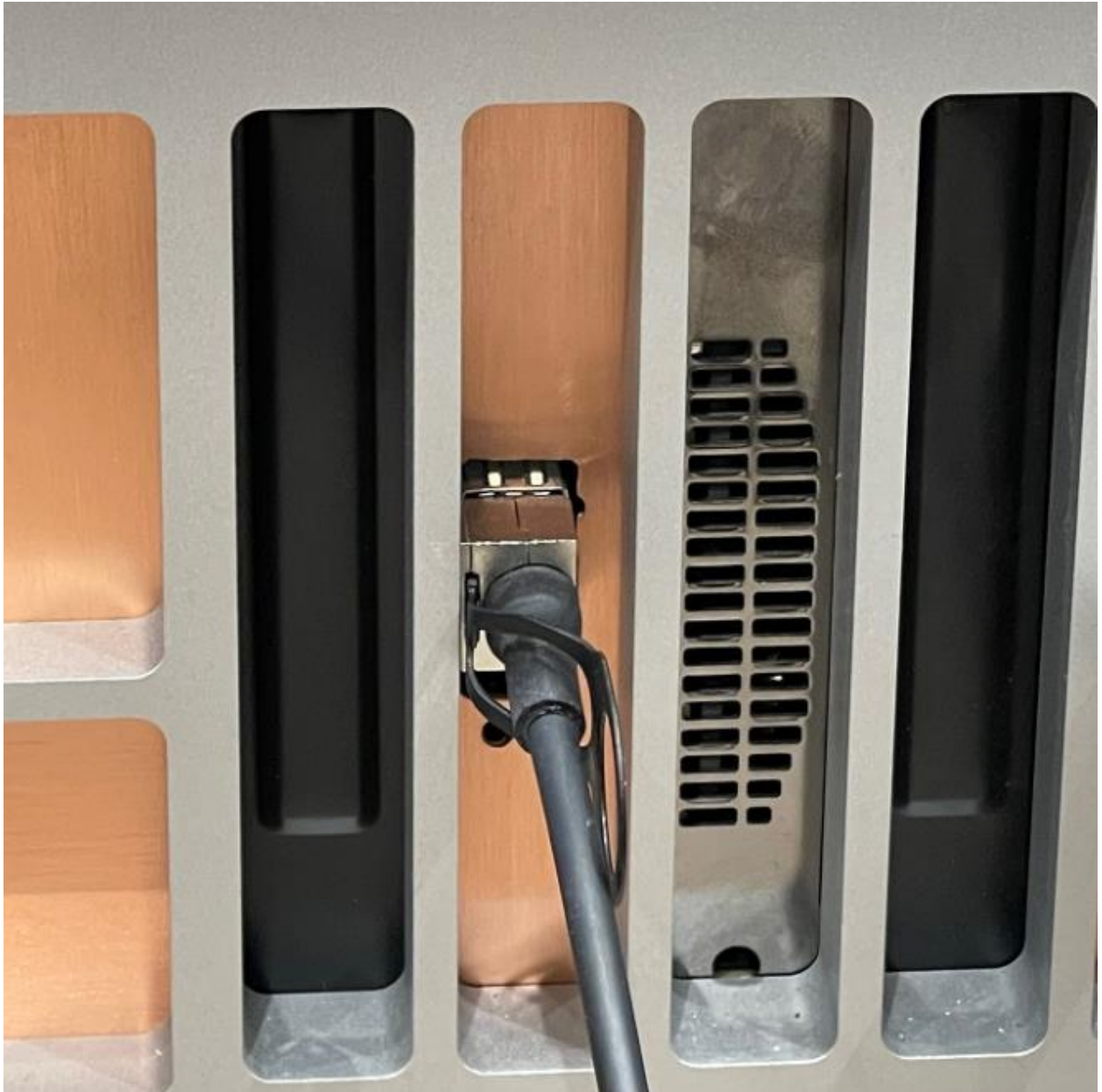
Above is a photo of the DAC Cable connected to a slot of the Extreme
